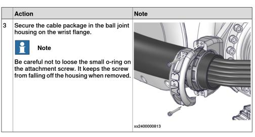
Fitting the cable package in upper arm tube
